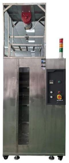
As a special equipment for testing the waterproof performance of the product in water, the product is tested by simulating the water environment at different depths, the performance of the product under flooded conditions, in particular the sealing performance of the shell. It is widely used in many fields such as electronics, automobile, medical, to ensure that the product can resist the intrusion of water in actual use, so as to ensure the safety and service life of the product.
