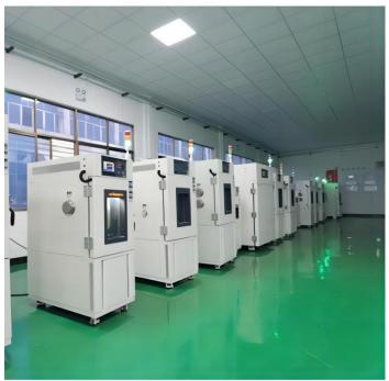
The humidity test can be conducted at the same time as the temperature test, so that the test effect is closer to the natural climate, simulating a worse natural climate, so that the reliability of the tested sample is higher.
